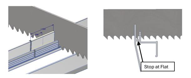
**Step 4.** Using a Utility Knife, scribe a line at the base of each leg.
