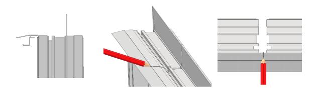
Step 3. Using a saw, or other cutting tool, cut two notches into the legs of the Drywall Return 1 inch apart (1/2" from each side of the centerline mark)
