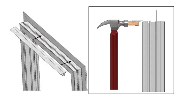
**Step 7.** Center drywall return on unit. Distance from edge of drywall return to edge of unit = 0.747"
