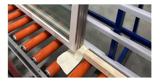
8) Using a caulk gun apply a 1/8" bead of silicone to the tape in the gap between the nail fins (see below). Fold the tape over the nail fin and make sure there are no bubbles. Press down on the gap between the nail fins to disperse silicone and minimize height of silicone addition. Remove extra tape on interior and exterior using a utility knife.
