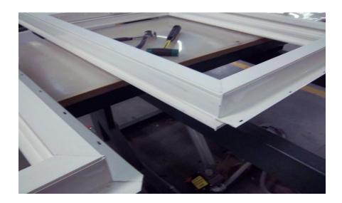
2) Clean out excess weld material at all 4 corners to be mulled using a chisel and a rubber mallet.
