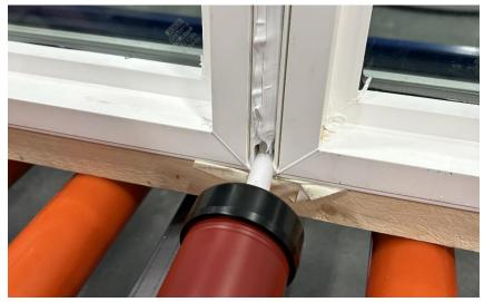
14) Apply a 1/8" bead of silicone to interior frame accessory groove.
