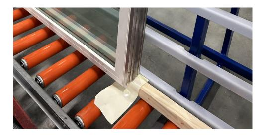
8) Using a caulk gun apply a 1/8" bead of silicone to the tape in the gap between the nail fins (see below). Fold the tape over the nail fin and make sure there are no bubbles. Press down on the gap between the nail fins to disperse silicone and minimize height of silicone addition. Remove extra tape on interior and exterior using a utility knife.
