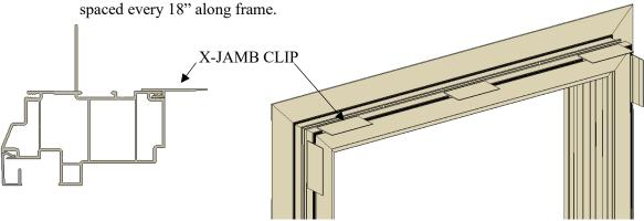
**Step 2.** Position jamb extension against the clips, as shown. Staple through the clip into the backside of the jamb extension with 3/8" x 1/2" staples
